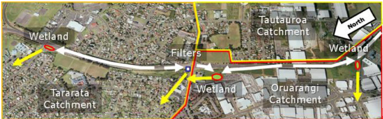
Figure 3.1. Original design proposing 3 stormwater wetlands and media filter cartridges (to treat stormwater pumped from the trench sump). White arrows indicate overland and piped flows into each device, yellow arrows indicate downstream flow into the public network.
