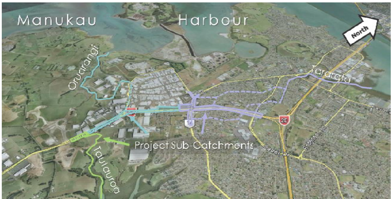
Figure 2.1. Aerial photograph providing indicative sub-catchment boundaries of the project area. Each of the three stream sub-catchments is outlined in a different colour. Where the stream network is piped, lines are shown as dashed.
