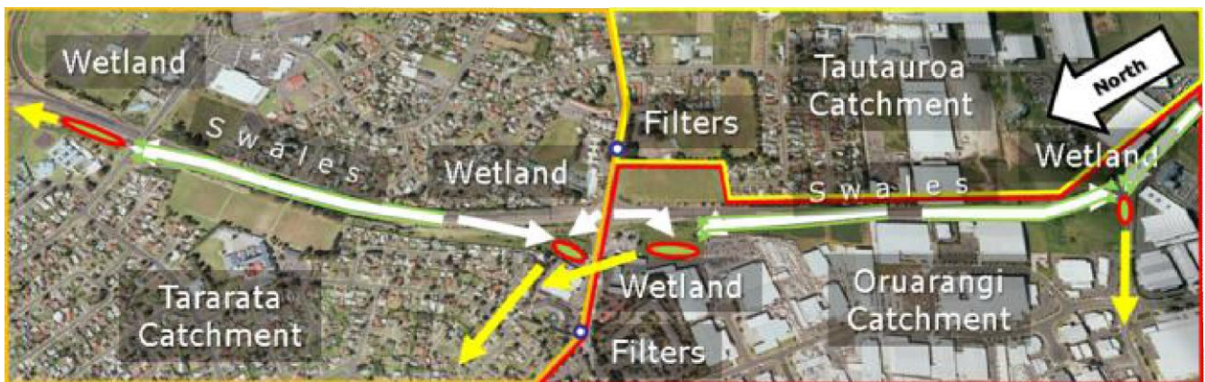
Figure 6.1. Consented design with 4 stormwater wetlands and media filter cartridges (to treat stormwater pumped from the local roads). Green arrows indicate roadside swales, white arrows indicate overland flows, yellow arrows indicate downstream flow into the public network.
