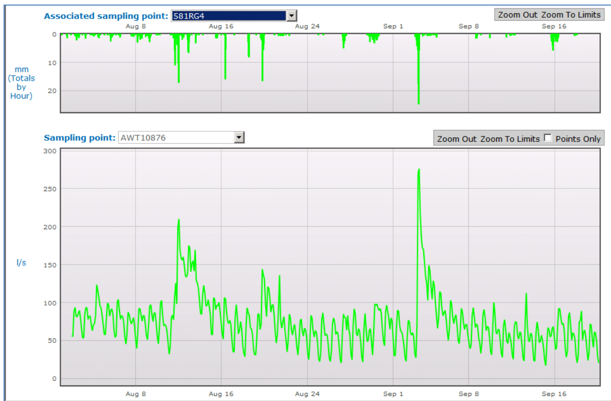
Figure 3: Network response to rainfall – quick rise after rain and slow regression indicates both inflow and infiltration issues
