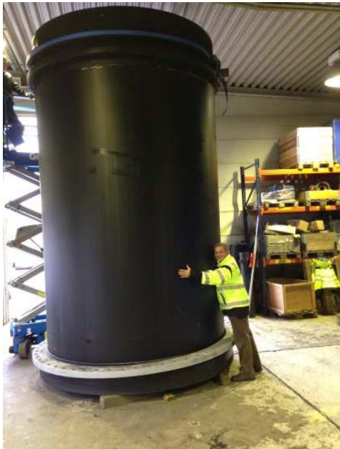
Photo 1 - The 2.5m diameter pipe section
