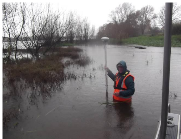
Photograph 1: Traditional river cross section profiles
