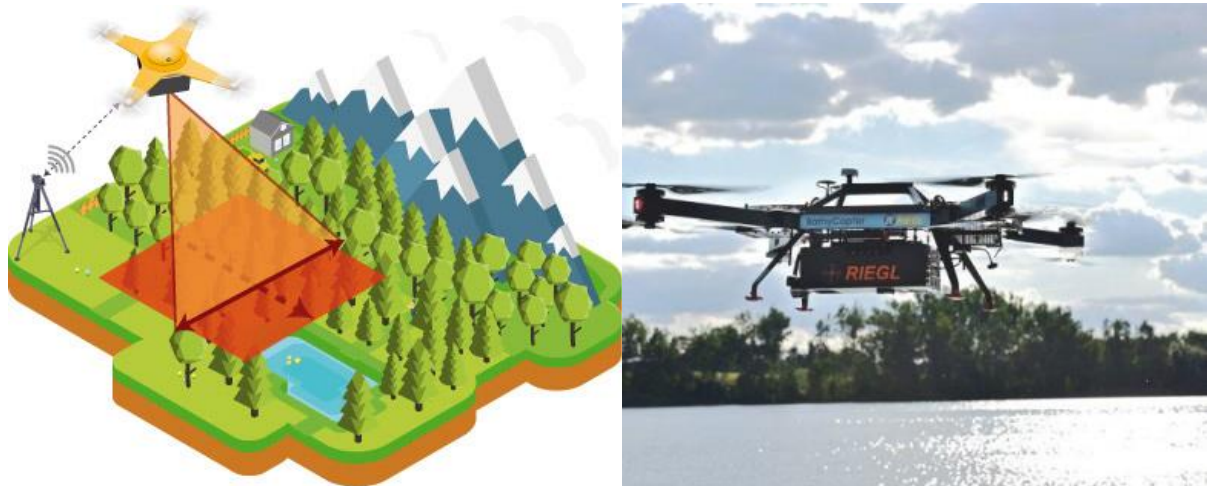
Figure 7: UAV fitted with Lidar
