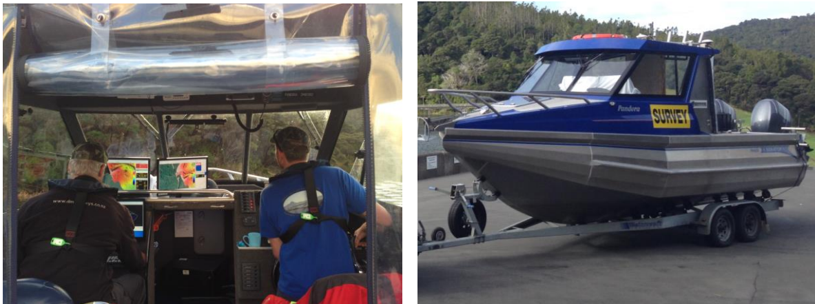
Photograph 2: 7m vessel with survey grade MBES fitted
