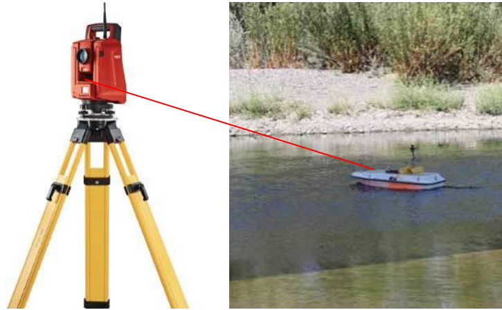
Figure 5: Robotic total station coupled with a USV
