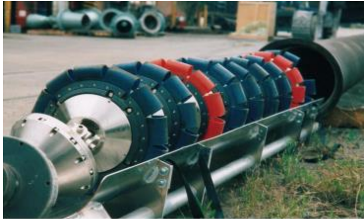
Figure 1 PCA introduced DN375 in-line inspection tool into Australia in 1998
