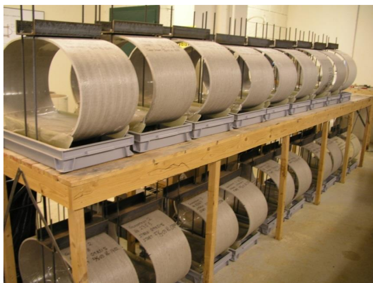
Photograph 2: Strain corrosion testing
