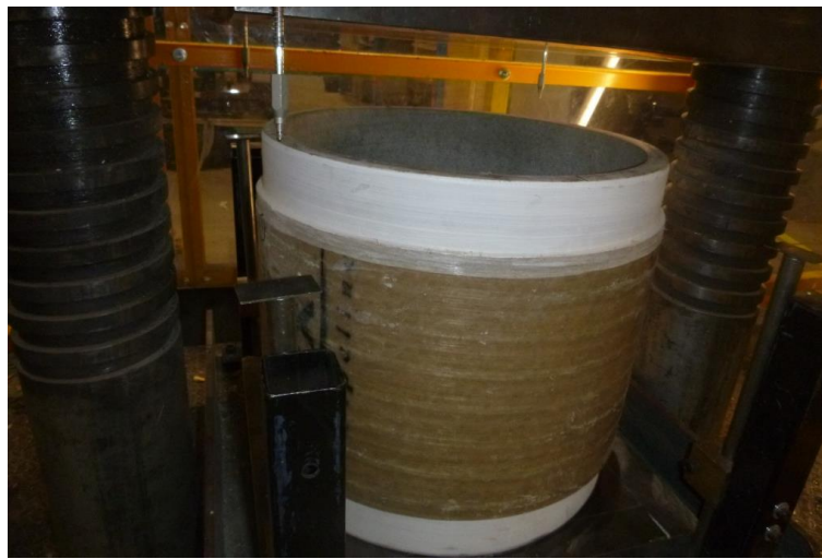
Photograph 3: Compression testing of pipe spool
