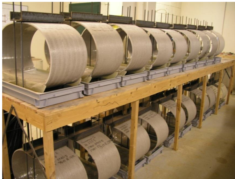
Photograph 3: Strain corrosion testing
