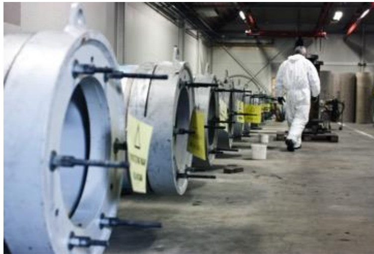
Photograph 4: Hydrostatic Design Basis (HDB) testing
