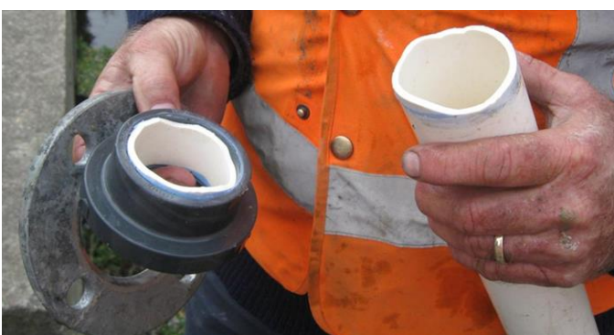
Photograph-1: View of fractured pipe and stub flange and DN 50 valve – where the stub flange was connected (Opus site records)
