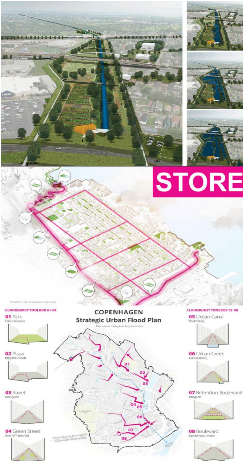
Figure 11: Potential Solutions to help manage extreme events across the three case studies. Top – Hollygrove District, New Orleans (GNO Urban Water Vision), Middle – Hoboken Town options for interconnected stormwater storage, New Jersey (OMA, 2014) and Bottom - Fredricksburg East and Vesterbro districts, Copenhagen (Ramboll, 2016).
