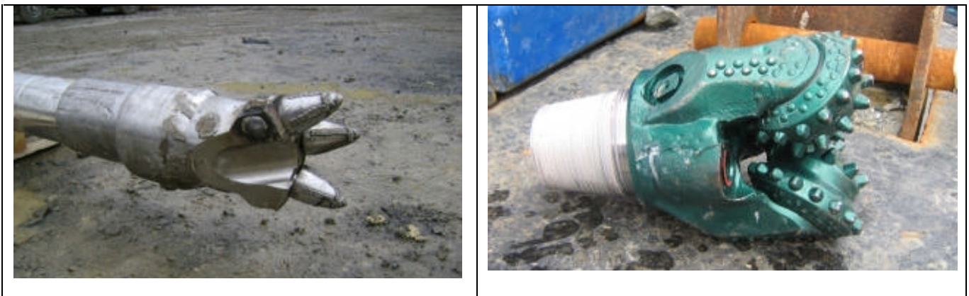
Photograph 7: Drill heads used for the pilot drill (Courtesy of Smythe Contractors)
