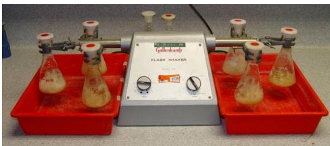
Photograph 1: Flask shaker used in batch testing of Ngakuru zeolites and NaCl solutions
