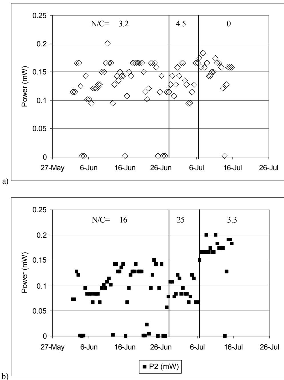
Figure 5: Impact of nitrogen limitation on (a) power density and (b) coulombic conversion efficiency
