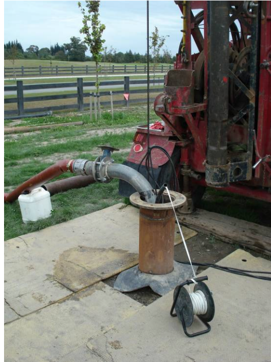
Figure 2. Typical pumping testing set up
