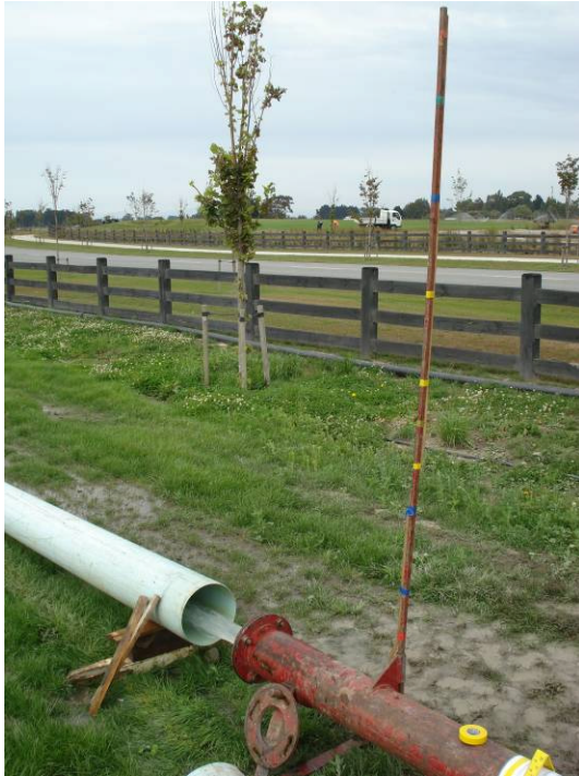
Figure 1. Pumping yield measured by orifice weir
