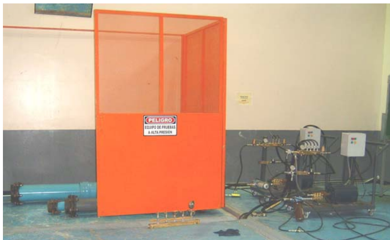
Internally restrained PVC pipe undergoing the million-cycle test
