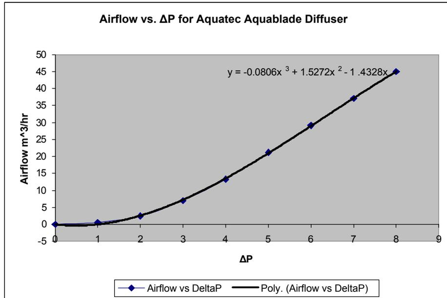
Figure 6: Airflow vs.  $\Delta P$  for Aquatec Aquablade Diffuser. The heavy black line is the Excel trend polynomial function (Poly.) that fitted the Aquatec data.
