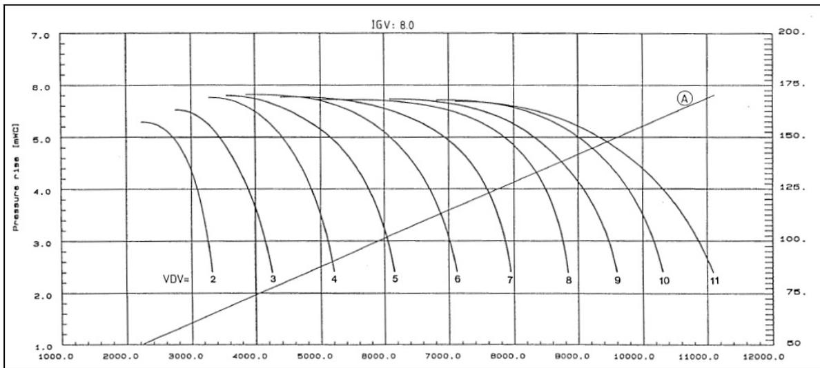
Figure 5: Fan Curves for different vane positions in a HV Turbo Blower
