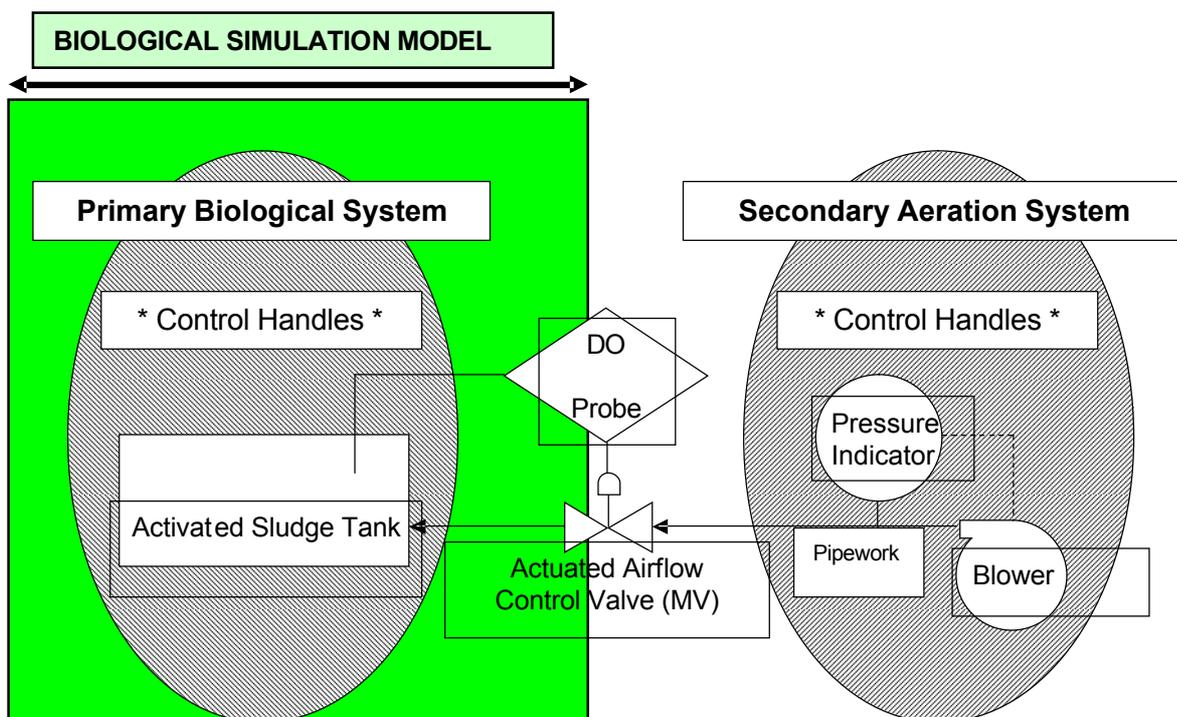
Figure 1: The two subsystems making up an activated sludge aeration system, showing the scope of standard biological simulators
