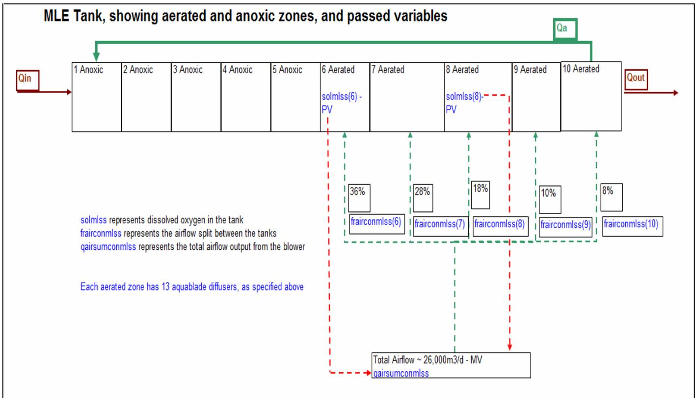
Figure 8: control basis of combined test model
