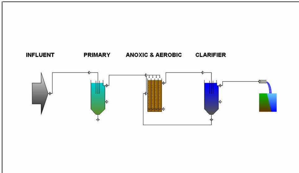
Figure 3: GPS-X test model
