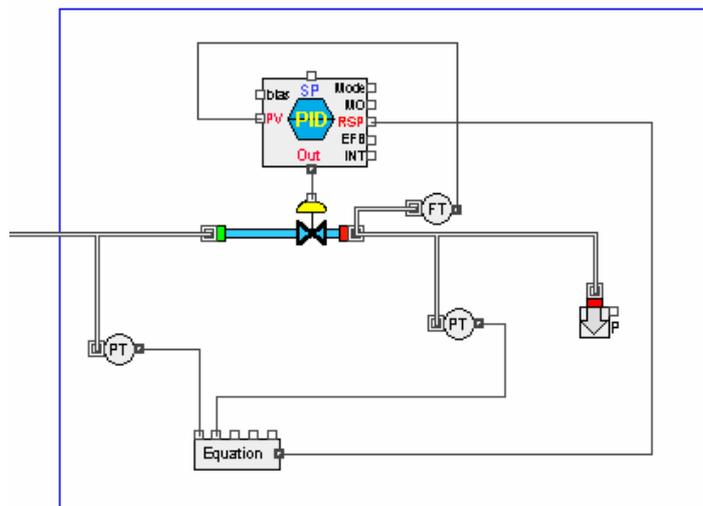
Figure 7: Final Diffuser Model. This model simulates the airflow and pressure drop of a diffuser using a linear valve and equation block.
