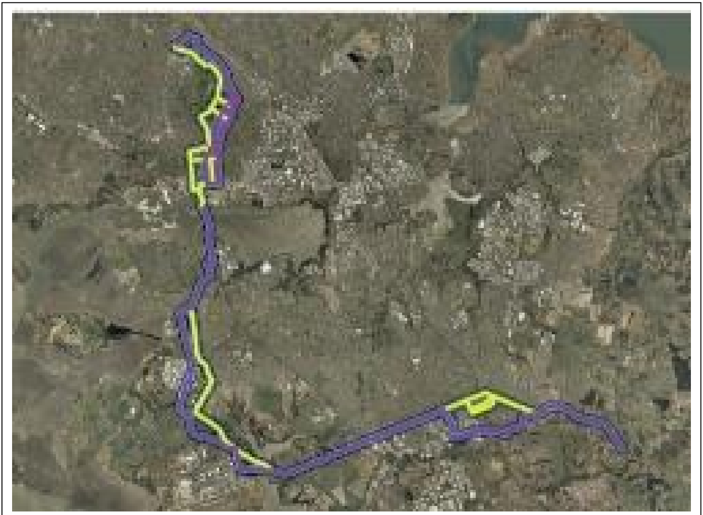
Figure 3 – Hunua 4 – Pipeline Route Options (as at May 2009)
