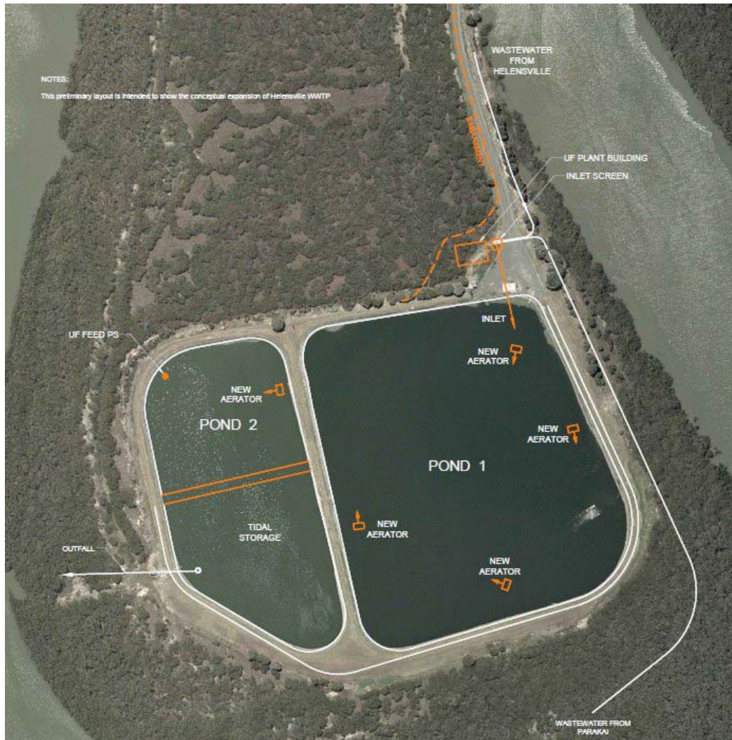
Figure 4: Helensville WwTP Plant Upgrades Layout Schematic Diagram
