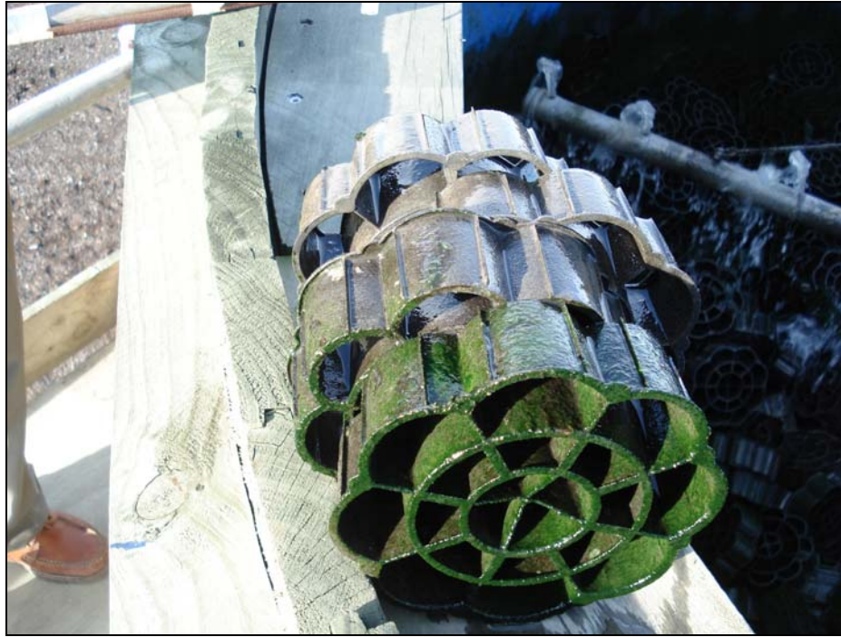
Photograph 3: Media collected from different depths of the BTF. Closest petal is from the top of the filter, showing strong algal growth.
