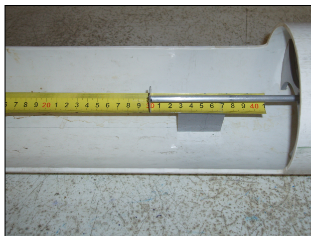
Figure 3: Measuring system on Percometer
