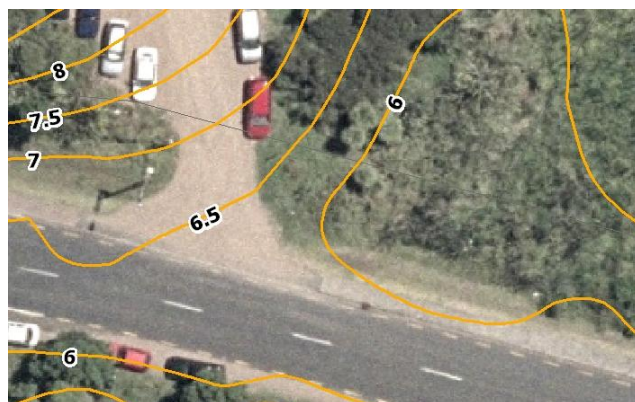
LIDAR 0.5m Contour and Aerial Photography
