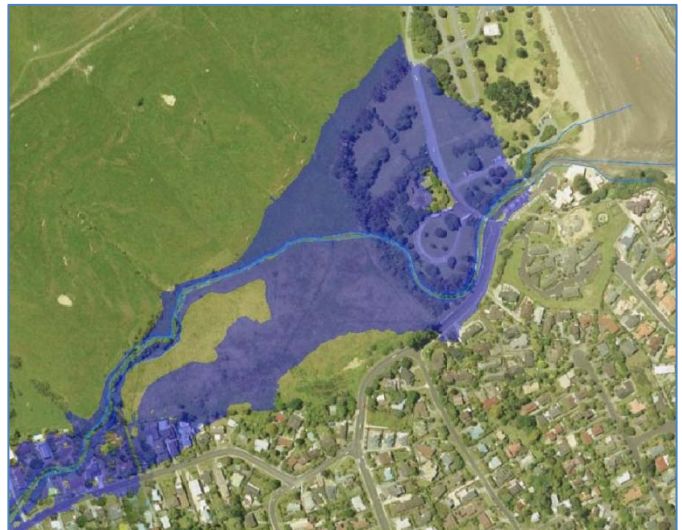
Figure 8: 100 Year Flood Extent Coupled 1d-2d Model
