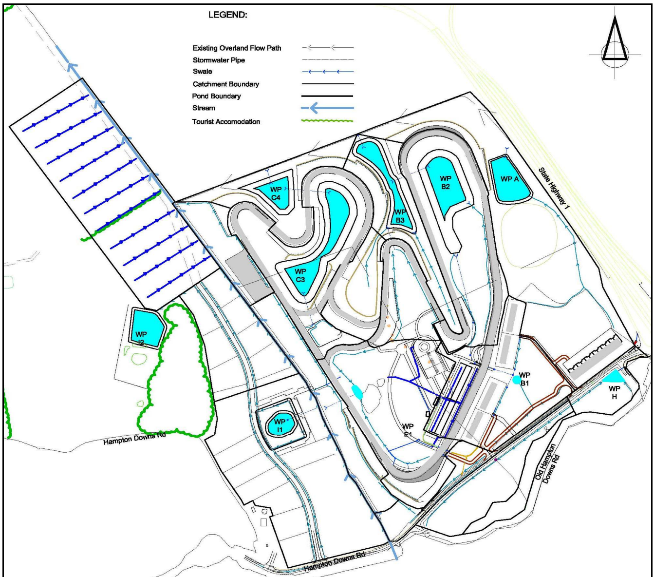
Figure 4: Stormwater Management Measures – Overview
