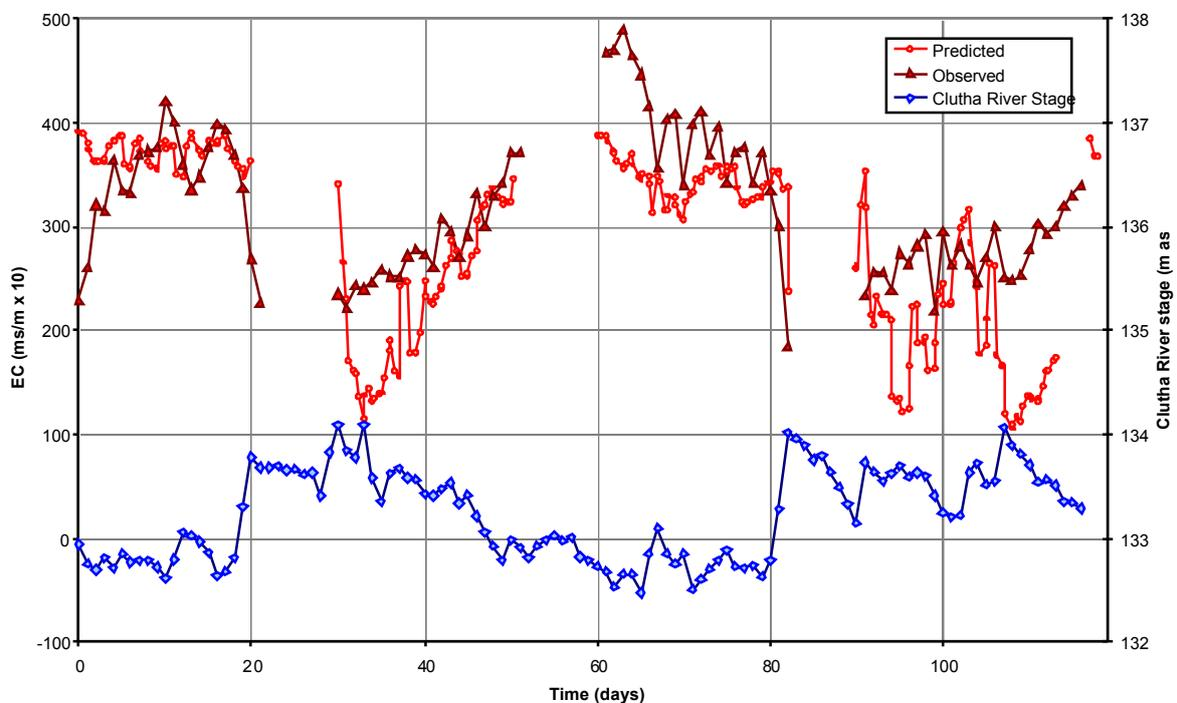
Figure 8: Observed and model wellfield EC response to river stage changes
