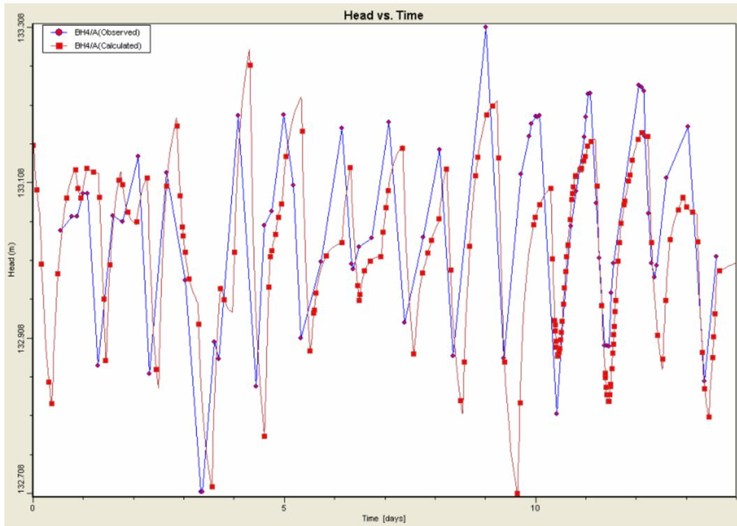
Figure 7: Observed and model well level response to river stage changes
