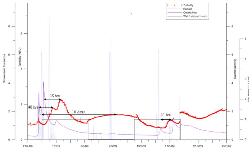
Figure 4: Turbidity Breakthrough Curves
