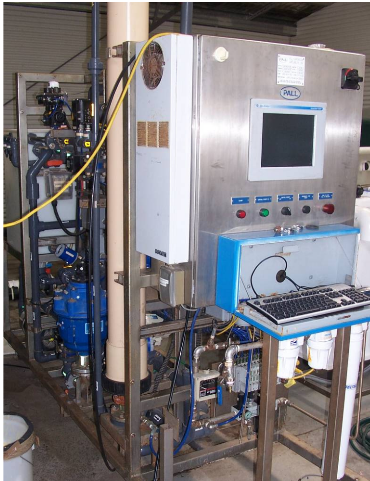
Photograph 3: Pall Single Module MF Pilot Skid
