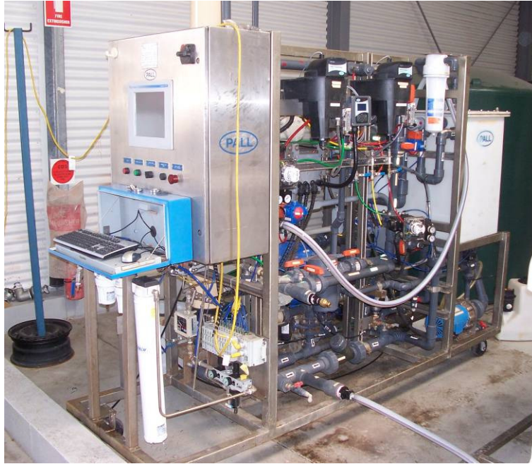
Photograph 4: Pall Single Module MF Pilot Skid
