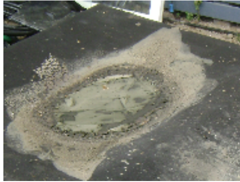
Figure 1: Drying algal biomass on non-woven geotextile drying rack
