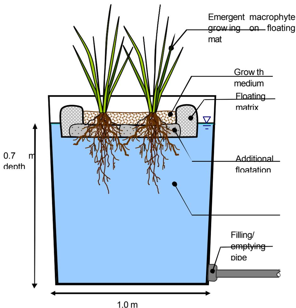
Figure 3: Cross-sectional diagram through mesocosm showing a planted  $0.6 \times 0.6 \text{ m}$  polyester floating matrix used in the experiments.
