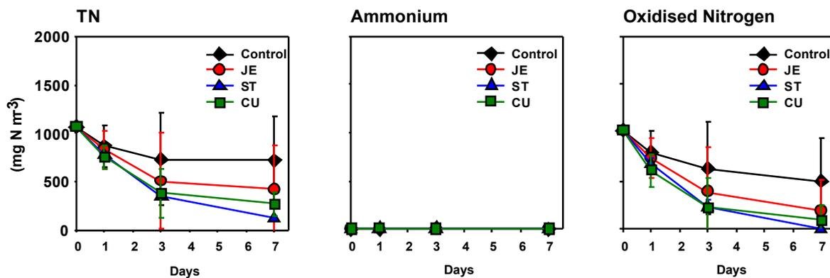
**Figure 10:** Mean concentration reduction of TN, ammonium and oxidised nitrogen during Experiment 3.
