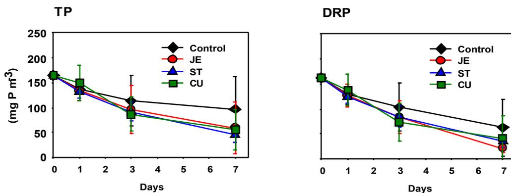
Figure 11: Mean concentration reductions of TP and DRP during Experiment 3.
