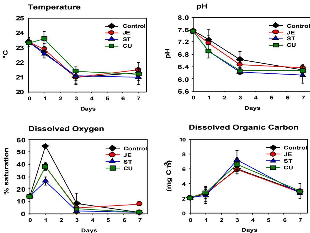
Figure 12: Mean Temperature, pH and DO, and DOC levels for FTWs and the controls during Experiment 4.
