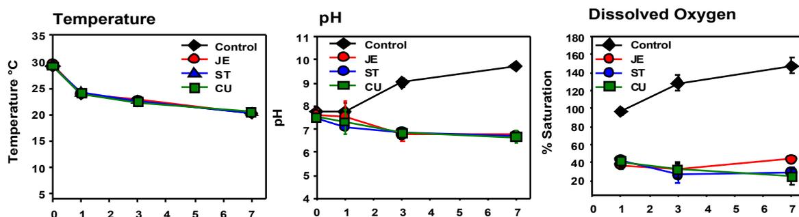
Figure 7: Temperature, pH and DO for FTW's and the control during Experiment 2.
