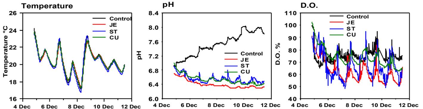
Figure 4: *Temperature, pH and DO for FTW's and the control during Experiment 1.*
