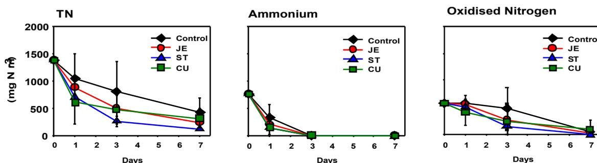
Figure 8: Mean concentration reductions of TN, ammonium and oxidised nitrogen during Experiment 2.
