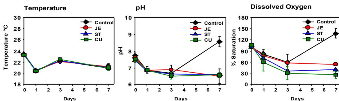
**Figure 9:** Mean Temperature, pH and DO levels for FTWs and the control during Experiment 3.
