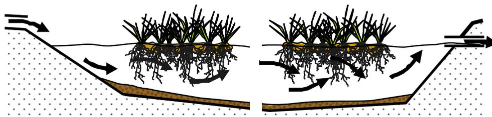
*Figure 1: Schematic longitudinal cross-section through a typical Floating Treatment Wetland system. Note that the water depth can vary appreciably in such a system without affecting plant growth (Source: Headley & Tanner, 2006).*
