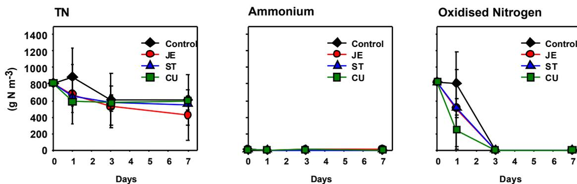
**Figure 13:** *Mean concentration reduction of TN, ammonium, and oxidised nitrogen during Experiment 4.*
