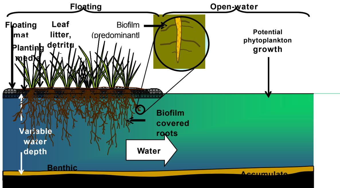
**Figure 2:** Cross-section of a typical floating treatment wetland showing main structural elements in comparison with an open-water lake or pond (Source: Headley & Tanner, 2006).
