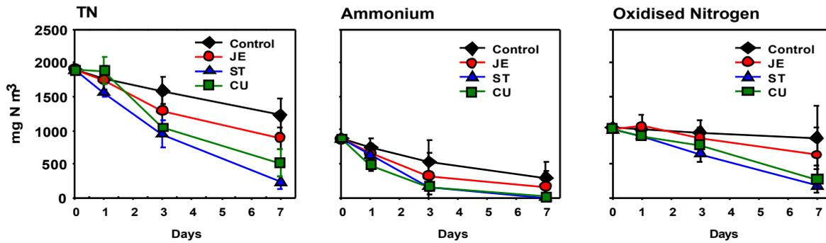
**Figure 5:** Mean concentration reduction of Total Nitrogen (TN), Ammonium ( $\text{NH}_4^+\text{-N}$ ), and Oxidised nitrogen-N ( $\text{NO}_x\text{-N}$ ) during Experiment 1 (error bars are one standard deviation).
