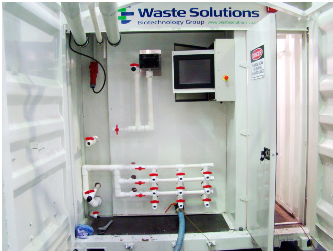
Photograph 2: The most recent containerized pilot plant, from the front. Touch panel HMI visible near centre. Door on the right allows secure access to the control system and the rest of the plant. This plant is fully controllable via internet connection.
