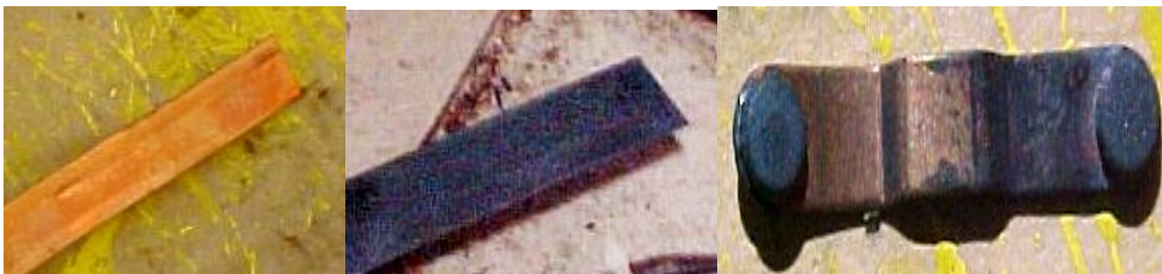
Photograph 2: H 2 S corrosion from WWTP plant. a, untarnished copper, b, corroded copper, c, silver contacts badly blackened
