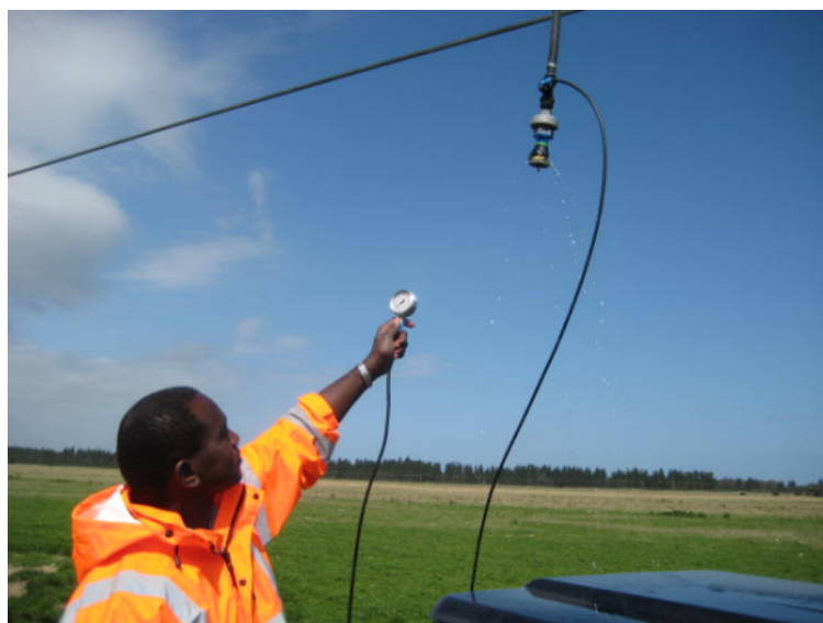
Figure 2: Pivot Pressure Measurement
