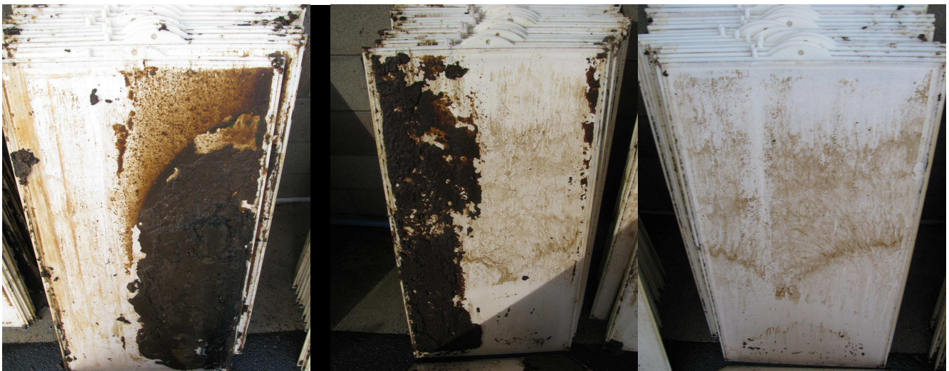
Photograph 3: Examples of spectrum of sludge caking observed
