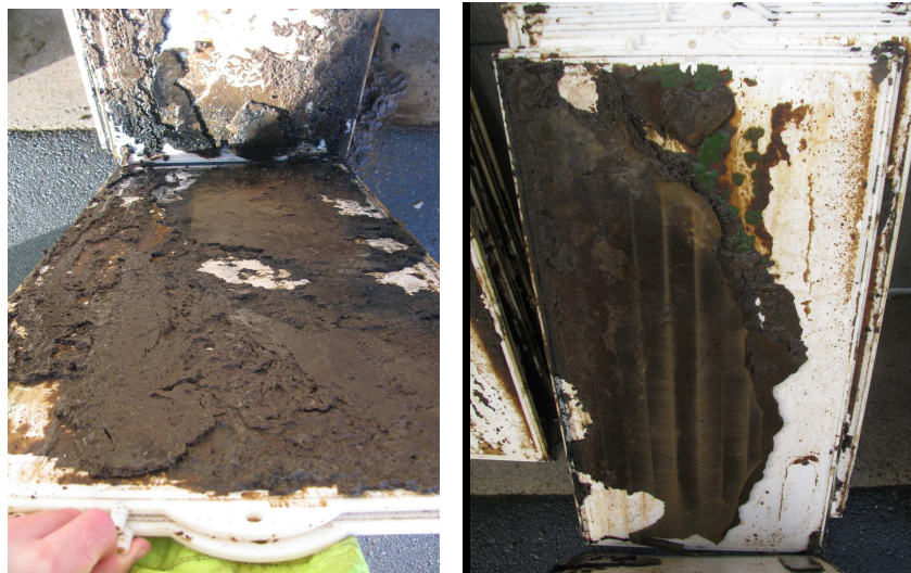
Photograph 3: Examples of spectrum of sludge caking observed
