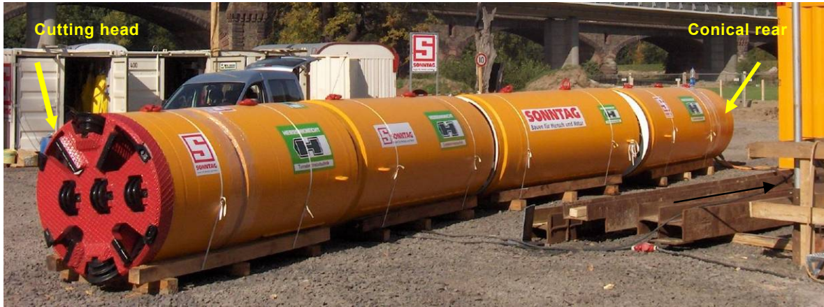
Figure 3: The Direct Pipe machine AVN1000XC for laying a 48"-pipeline.
