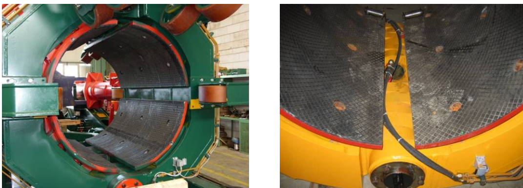
Figure 6: Clamping unit of the Pipe Thruster with clamping inserts with vulcanized contact rubber.
