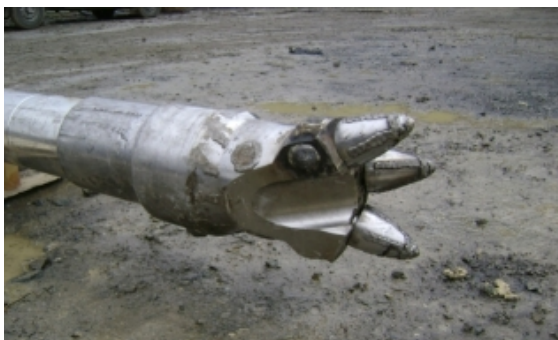
Picture 5: Drill heads used for the pilot drill (Courtesy of Smythe Contractors)
