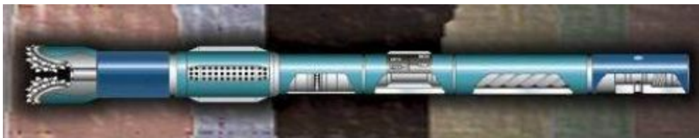
Picture 4: The Mud Motor (Courtesy of Kalsi Engineering)
