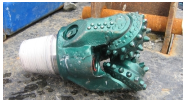
Picture 5: Drill heads used for the pilot drill (Courtesy of Smythe Contractors)
