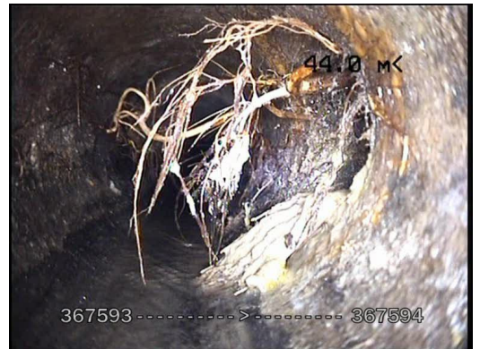
Figure 10: RI should be removed before LJR
