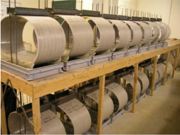
Figure 1 Pipe samples under chemical resistance testing
