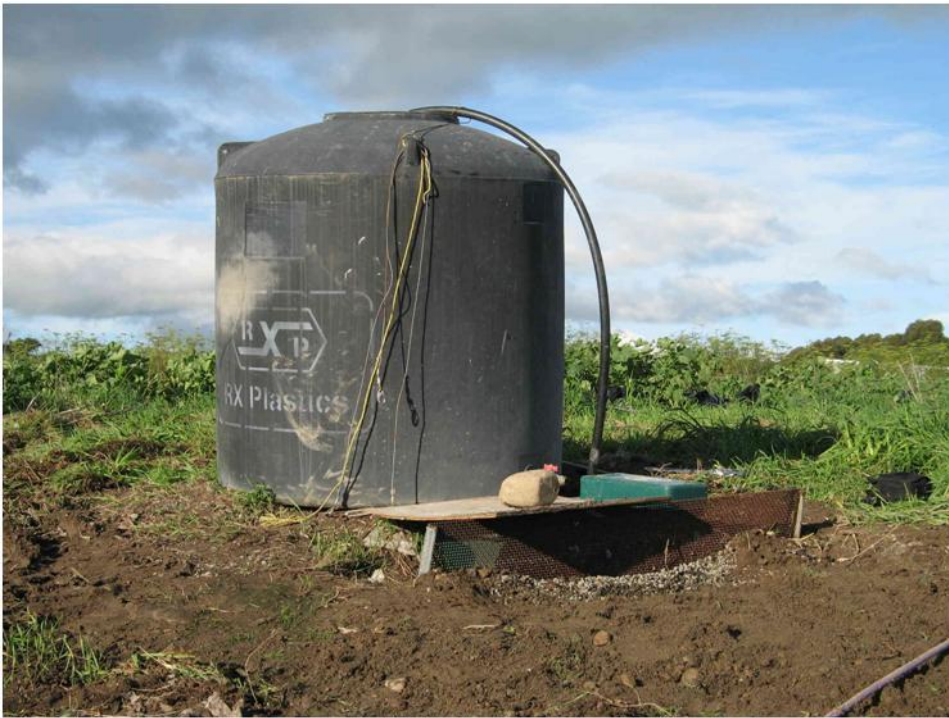
Figure 9 Header tank for dose loading of viruses
