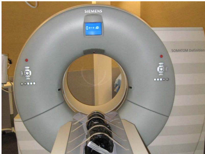
Figure 3-5 CT Scanner (Siemens SOMATOM) Loaded with AC Pipe Samples
