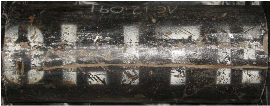
B2-1: Early Fibrolite pipe (circa 1954), bitumen dipped: - White stencilling reads “Fibro OLITE pressure pipe”.
