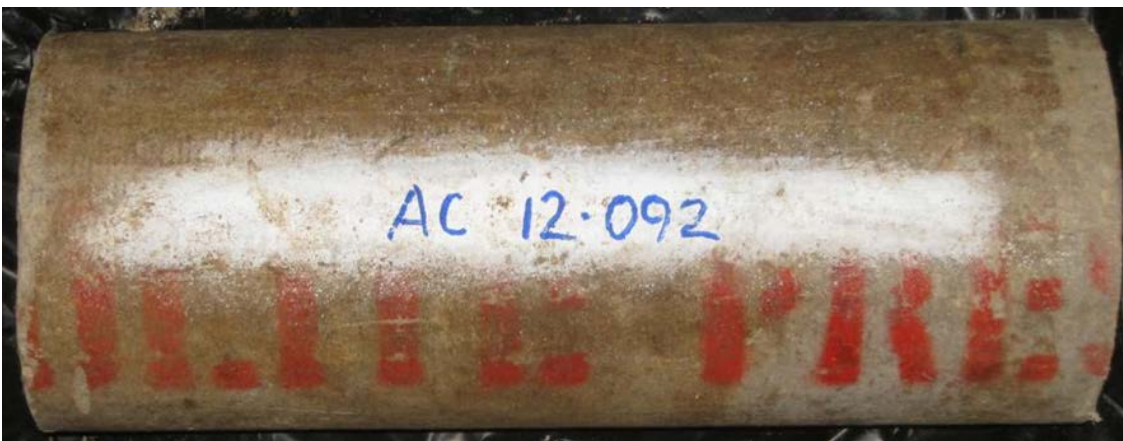
B2-2: Fibrolite pipe, circa 1961, - Red stencilling reads “Fibro OLITE PRES sure pipe”.
