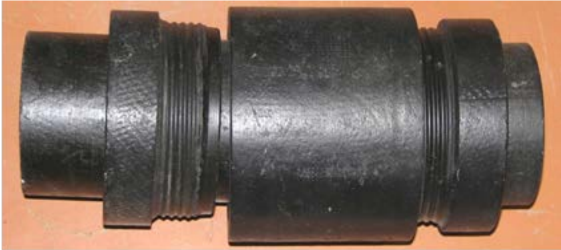
B1-3: Photograph of Everite screw joint disassembled.
